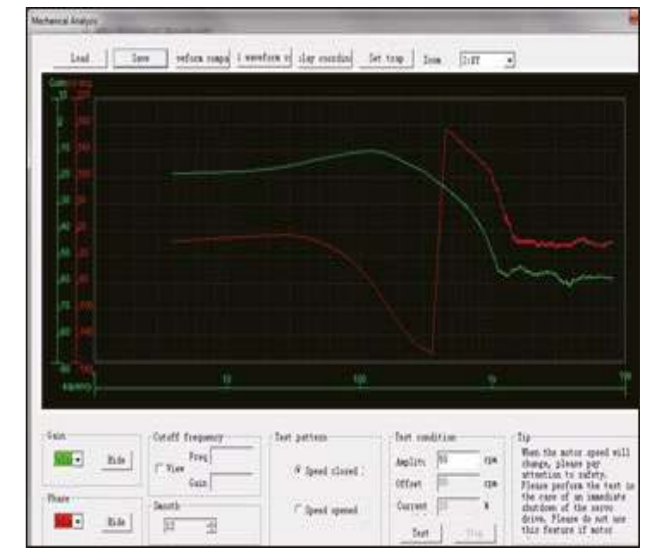
Mechanical analysis to diagnose natural frequency of system
